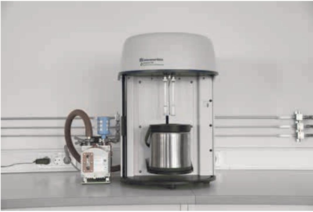
Figure 1: Duo 1.6 rotary vane pump from Pfeiffer Vacuum in use on a surface analyzer from Micromeritics GmbH.
